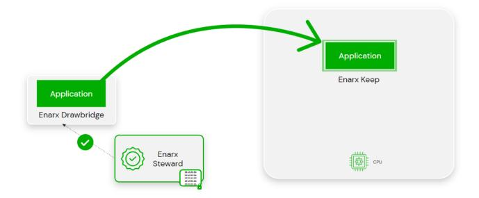
If the Attestation service validates the measurement, the application can be safely deployed.
