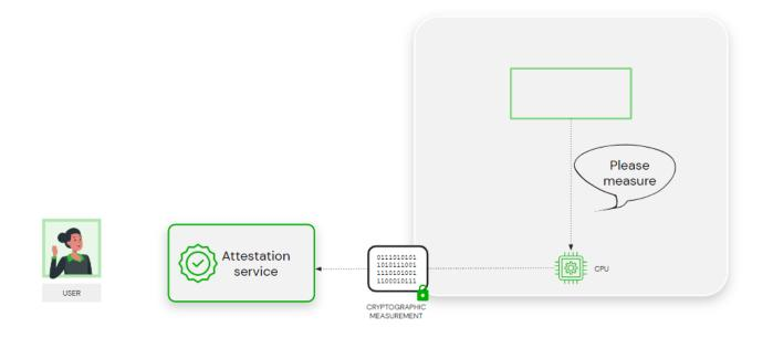
The TEE instance requests a measurement from the CPU, which is passed to an Attestation service
